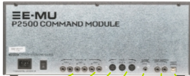
Sub Analog Outputs Main Analog Outputs MIDI In MIDI Out/Thru A & B S/PDIF Output Footswitch Inputs 1 & 2 USB Connector
